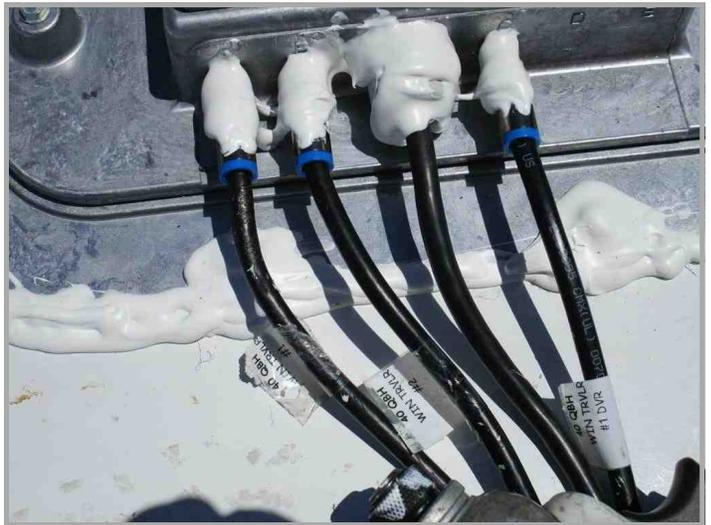
All connected and ready for the weather. Don't forget to apply dicor to the antenna edge at the roof and over all the screws to the roof.
