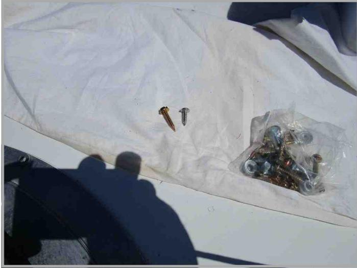
The gold screws came with the Trav'ler. I purchased 5/8" stainless steel after speaking to the Tiffin factory about the duct and roof areas.
