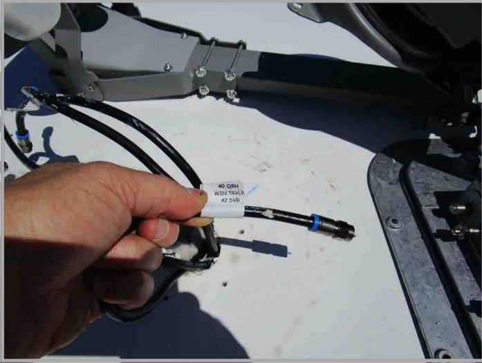
A 4th coax cable, where only 3 are used for Dish HD. I pushed this cable back into the ceiling area when I was dry fitting the antenna.
