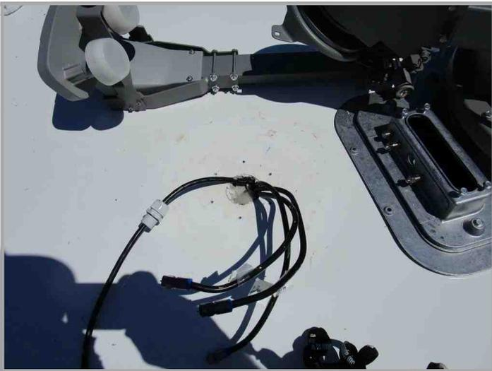
Now I have 3 coax cables and 1 data line to connect to the Trav'ler. One can see the proximity of the antenna to the cable openings.
