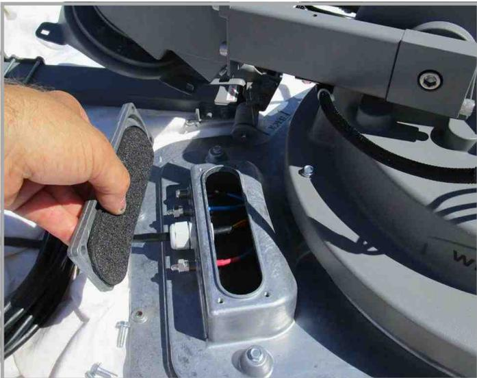
The Trav'ler antenna comes with an installed data cable that must be replaced with the Tiffin pre-wired data cable. Remove this plate.
