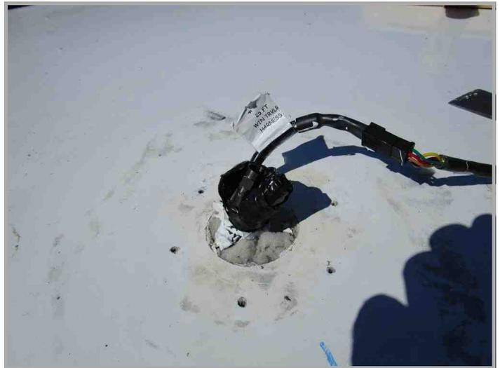
Cleanup almost done. I think I used alcohol and lots of TLC to remove the remaining dicor. Notice the coax wiring ball in black tape.
