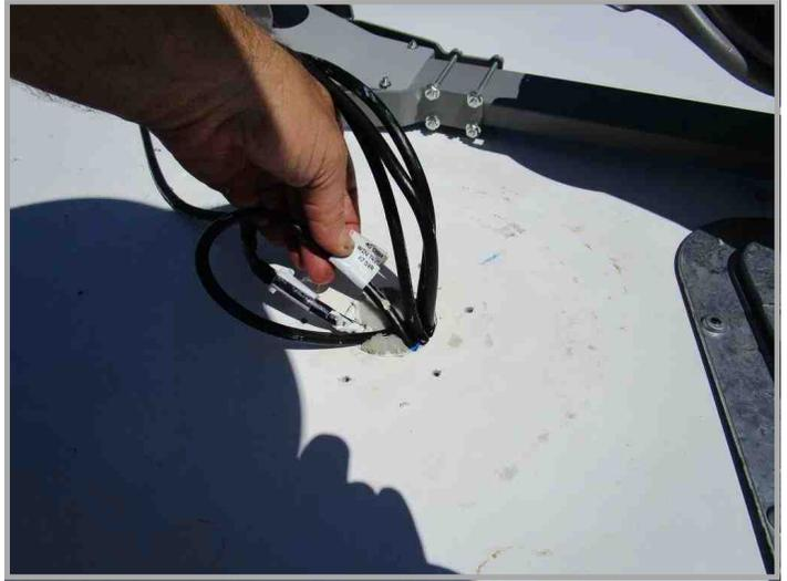
The cable duct area has foam rubber. Push the cable pass the foam than reposition the foam rubber. I filled the top area in with dicor.
