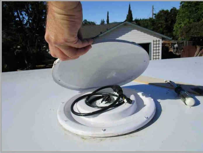
Removing the top half piece of the factory pre-wiring dome. Notice this is only the Trav'ler data cable.
