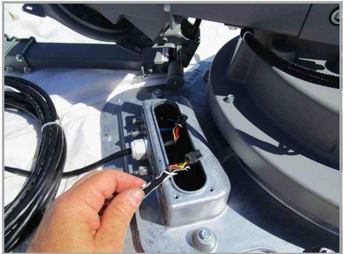
Here I am holding the Tiffin pre-wired data cable after I reached into the opening and disconnected the Trav'ler supplied data cable.
