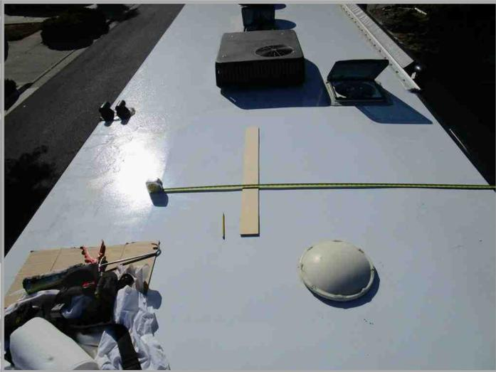
Here the general location over the bedroom slideout. The white fiberglass dome houses the factory Trav'ler pre-wiring.
